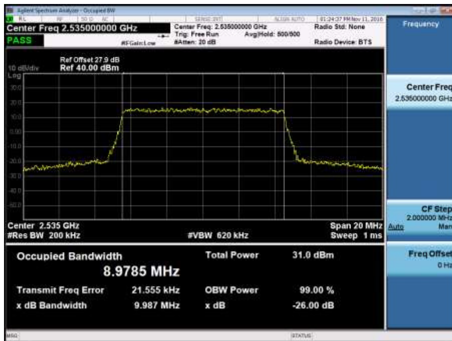
BAND7. Occupied Bandwidth Plot (10MHz Ch.21100 QPSK RB 50)
