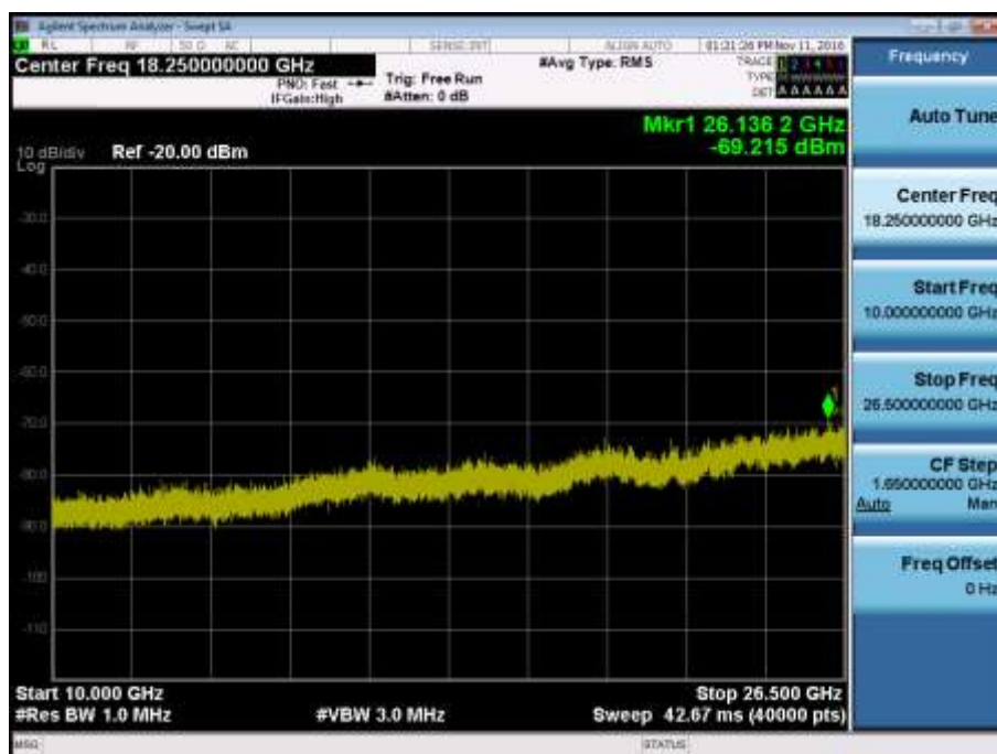
BAND7. Conducted Spurious Plot 2 (5MHz Ch.21100 QPSK RB 1, Offset 0)
