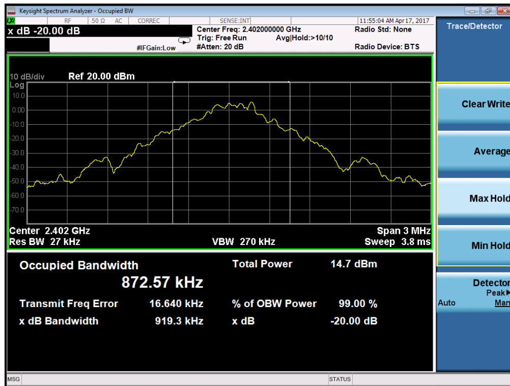
Plot 7-1. 20dB Bandwidth Plot (Bluetooth, 1Mbps – Ch. 0)
