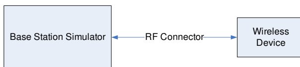
Figure 9-2 Power Measurement Setup
