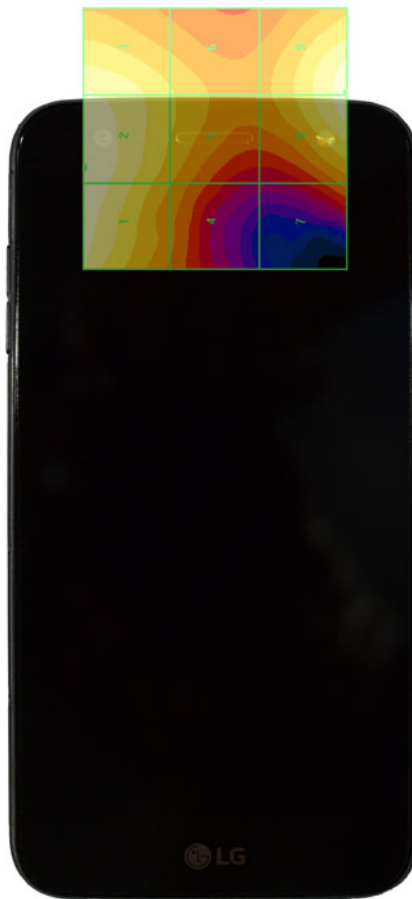
Figure 17-4 E-Field WD Scan overlay
