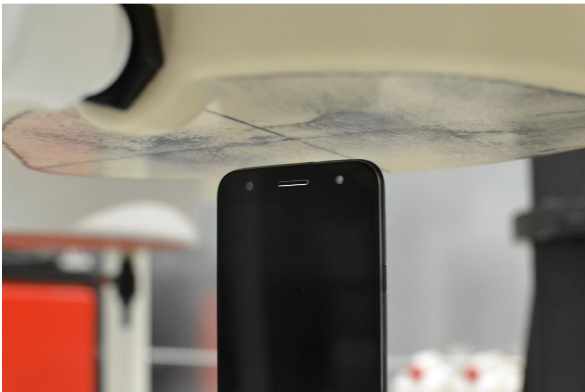
SAR Test Setup Photo 9 – Top Edge at 10 mm
