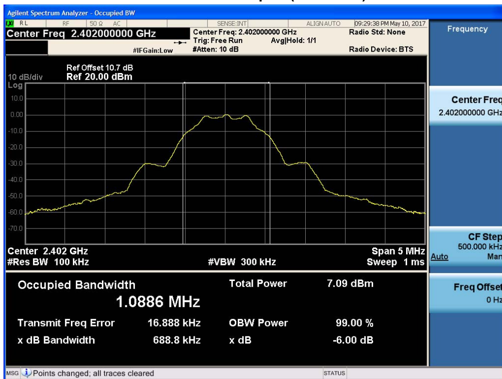
6 dB Bandwidth plot (Low-CH 0)
