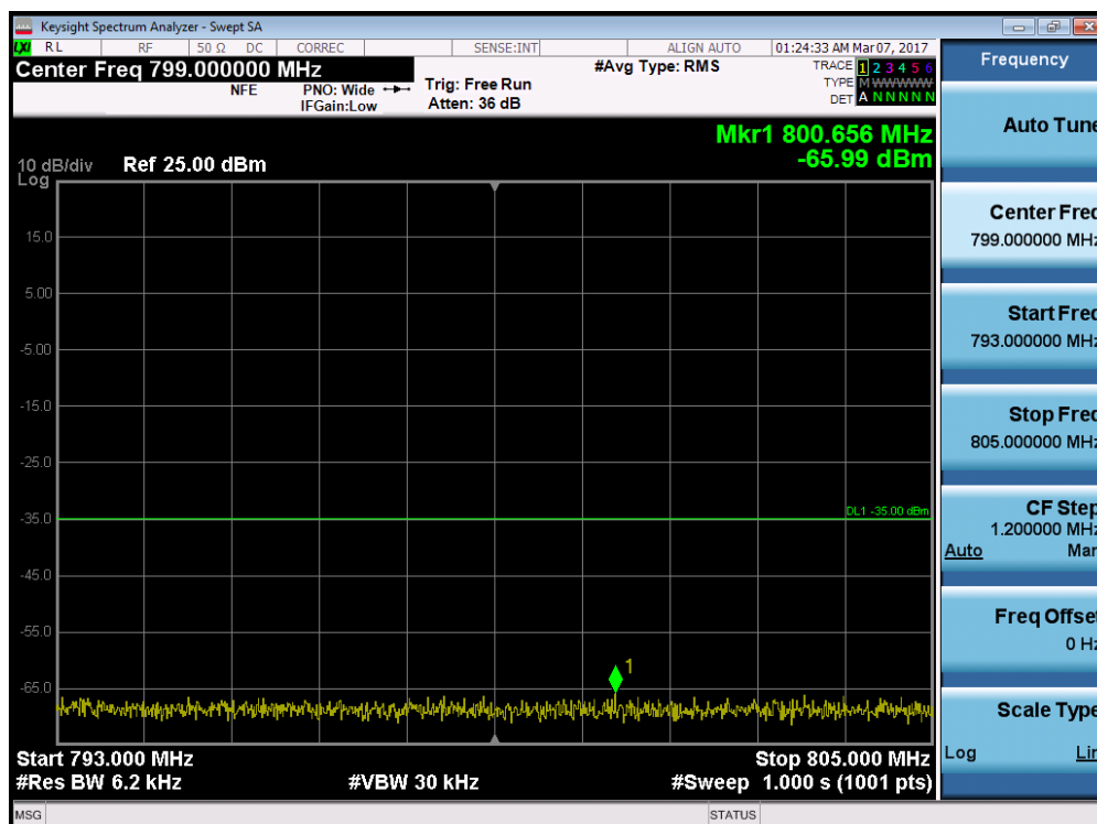
Plot 7-140. Upper Emission Mask Edge Plot (Band 13 – 10.0MHz QPSK – RB Size 50)
