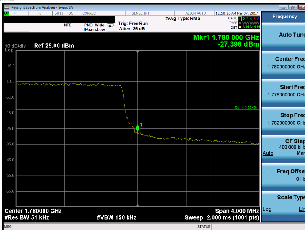
Plot 7-185. Upper Band Edge Plot (Band 66 – 5.0MHz QPSK – RB Size 25)
