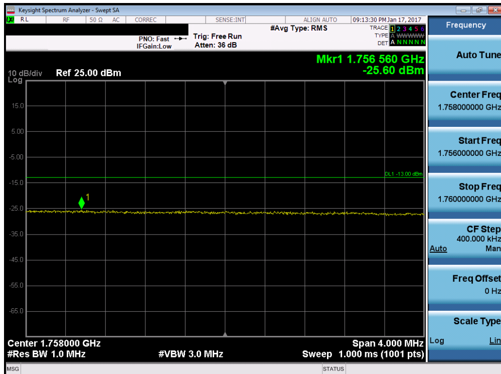
Plot 7-170. Upper Extended Band Edge Plot (Band 4 – 15.0MHz QPSK – RB Size 75)
