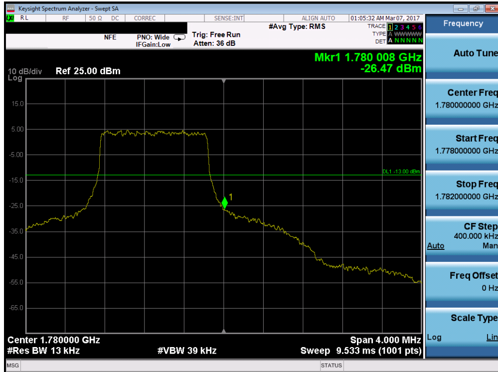
Plot 7-177. Upper Band Edge Plot (Band 66 – 1.4MHz QPSK – RB Size 6)
