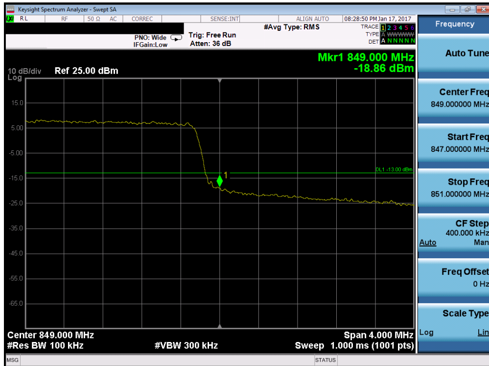
Plot 7-148. Upper Band Edge Plot (Band 5 - 5.0MHz QPSK - RB Size 25)
