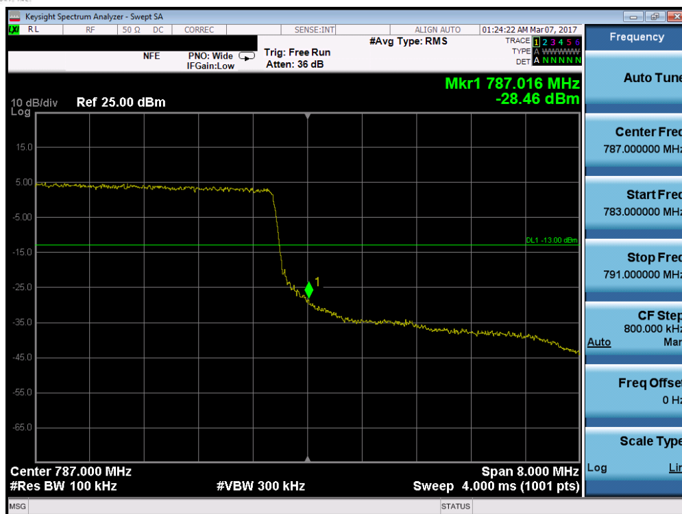
Plot 7-139. Upper Band Edge Plot (Band 13 – 10.0MHz QPSK – RB Size 50)
