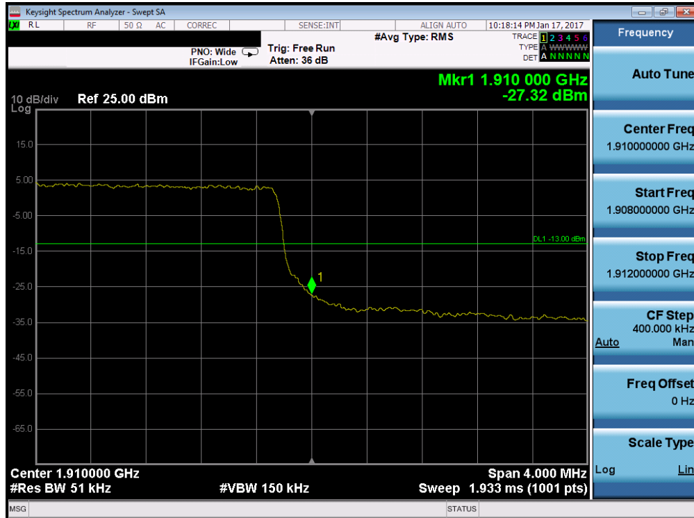
Plot 7-209. Upper Band Edge Plot (Band 2 - 5.0MHz QPSK - RB Size 25)
