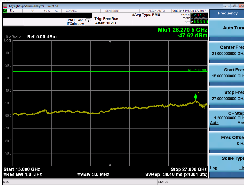
Plot 7-117. Conducted Spurious Plot (Band 7 – 10.0MHz QPSK – RB Size 1, RB Offset 0 – Low Channel)
