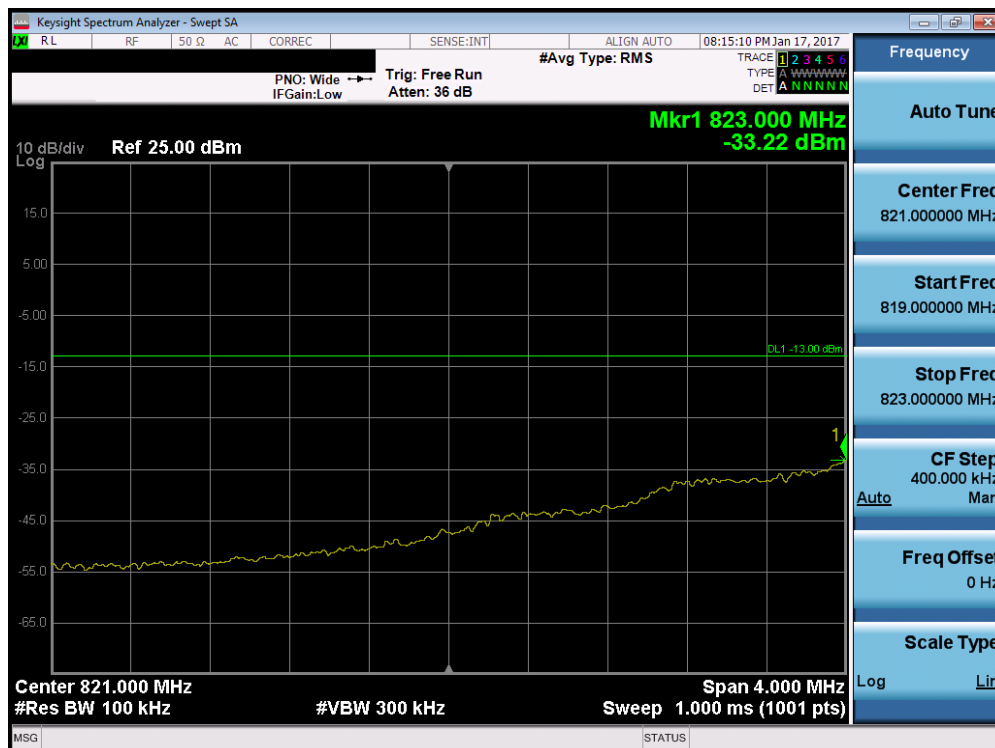
Plot 7-142. Lower Extended Band Edge Plot (Band 5 – 1.4MHz QPSK – RB Size 6)
