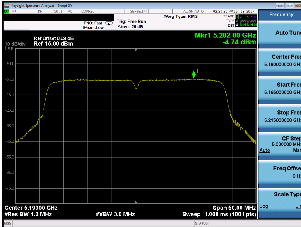
Plot 7-44. Power Spectral Density Plot (40MHz BW 802.11n (UNII Band 1) – Ch. 38)
