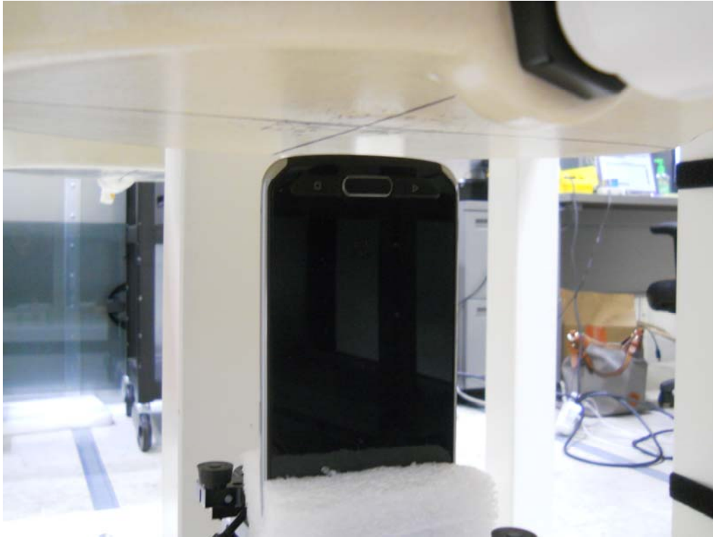
SAR Test Setup Photo 9: Bottom Edge at 1.0 cm
