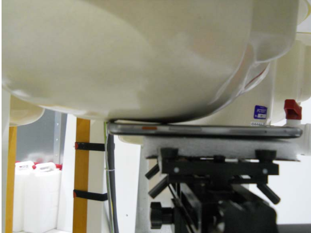
SAR Test Setup Photo 1: Right Cheek
