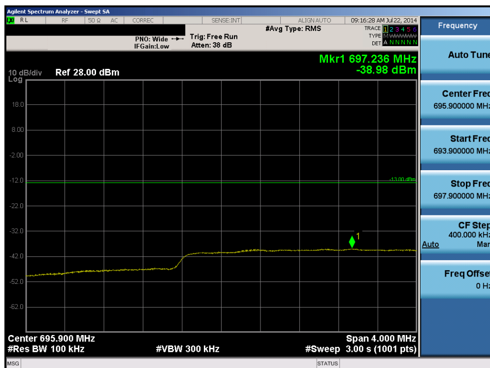
Plot 6-58. Lower Extended Band Edge Plot (Band 17 – 10.0MHz QPSK – RB Size 50)
