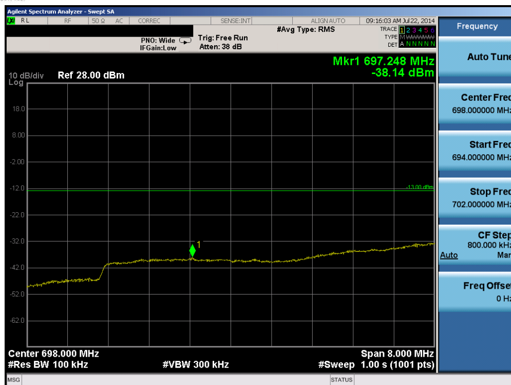
Plot 6-57. Lower Band Edge Plot (Band 17 – 10.0MHz QPSK – RB Size 50)
