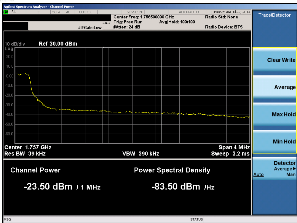
Plot 6-63. Upper Extended Band Edge Plot (Band 4 – 5.0MHz QPSK – RB Size 25)
