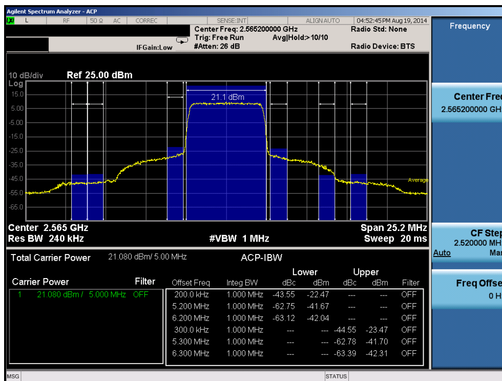
Plot 6-94. Upper ACP Plot (Band 7 – 5.0MHz QPSK – RB Size 25)
