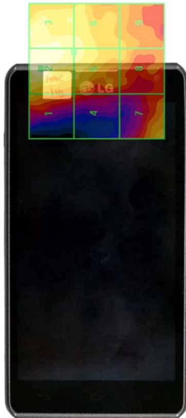
Figure 17-4 E-Field WD Scan overlay
