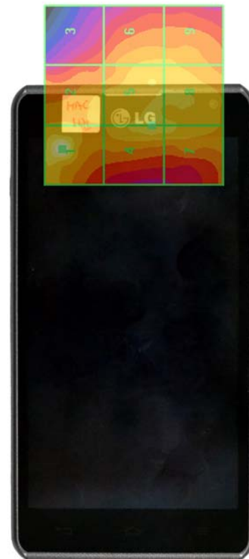
Figure 17-5 H-Field WD Scan overlay
