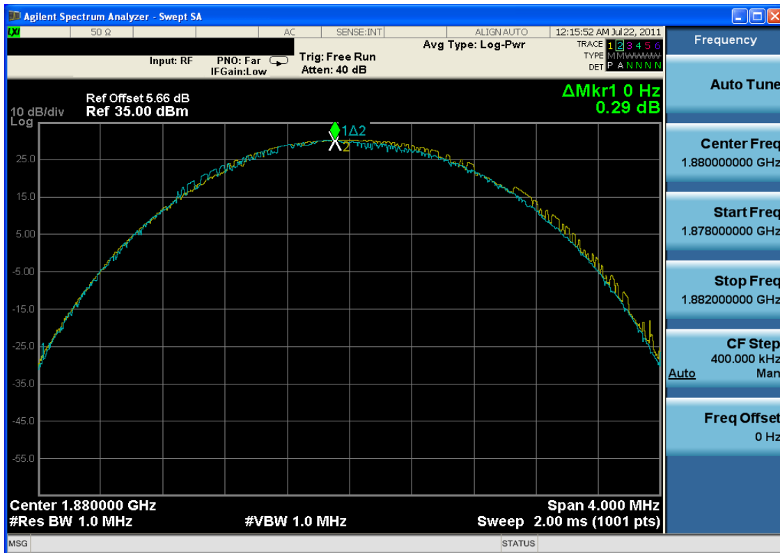
Plot 7-22. Peak-Average Ratio Plot (EDGE1900 Mode – Ch. 661)
