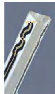
Figure 3.3 Probe Thick-Film Technique
