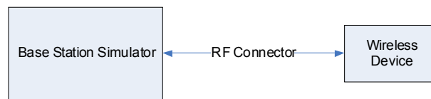
Figure 11-1 Power Measurement Setup
