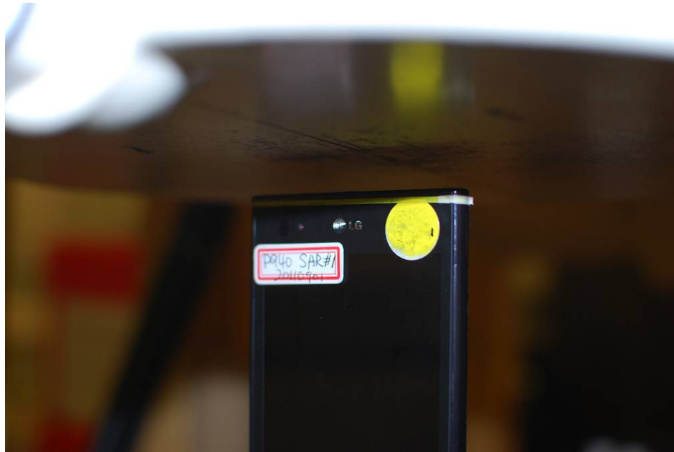
SAR Test Setup Photo 7 – Top at 1.0 cm
