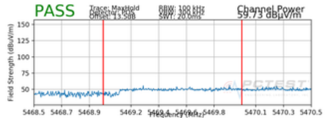
Plot 7-97. Radiated Lower Band Edge Plot (Peak – UNII Band 2C)
