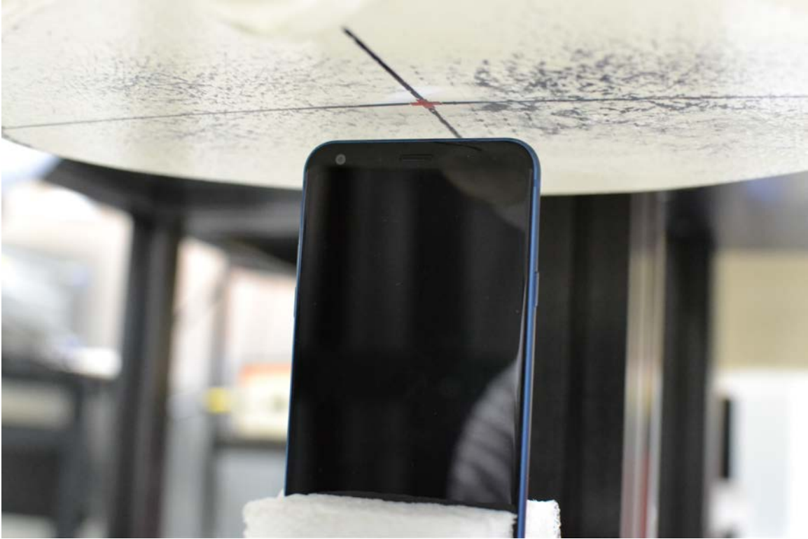
SAR Test Setup Photo 7: Top at 1.0 cm
