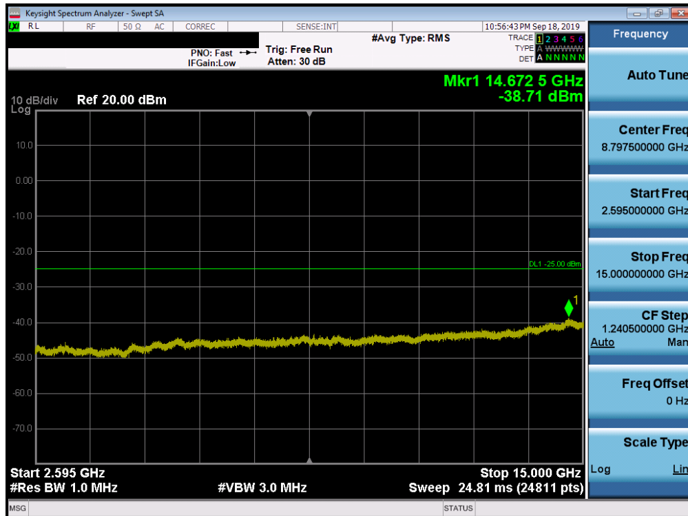
Plot 7-161. Conducted Spurious Plot (Band 7 - 20.0MHz QPSK - RB Size 1, RB Offset 0 - High Channel)
