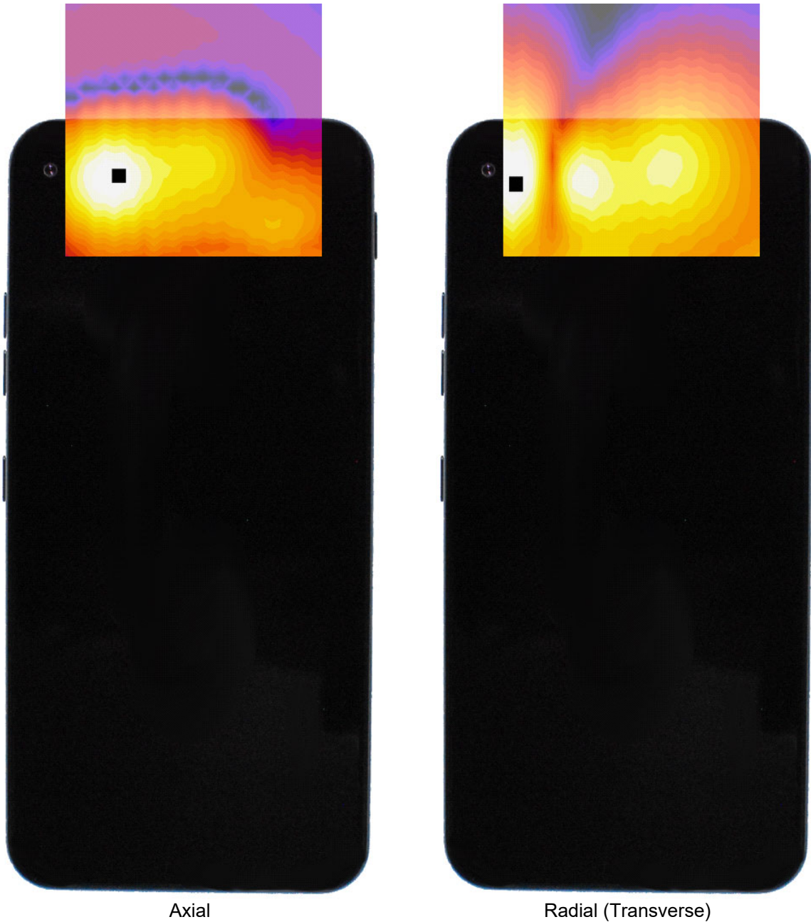
Figure 16-3 T-Coil Scan Overlay Magnetic Field Distributions
