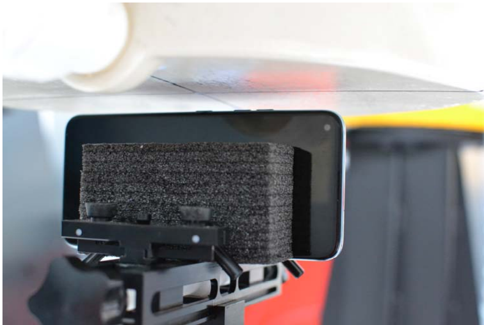
SAR Test Setup Photo 10: Left at 10 mm
