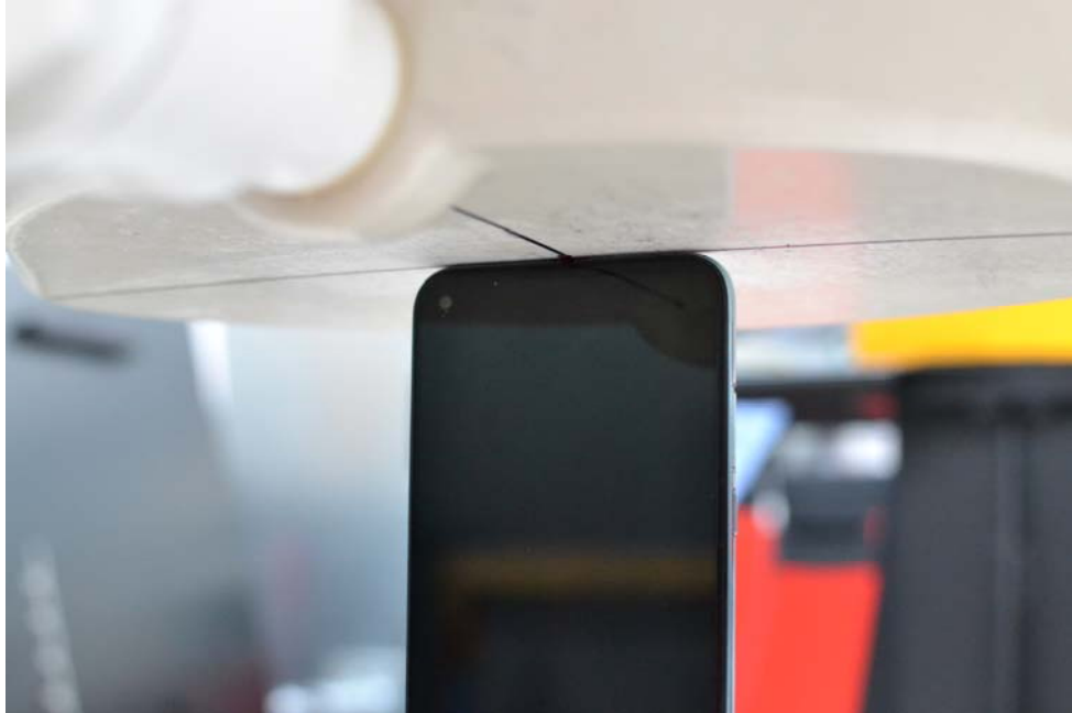
SAR Test Setup Photo 14: Top at 0 mm
