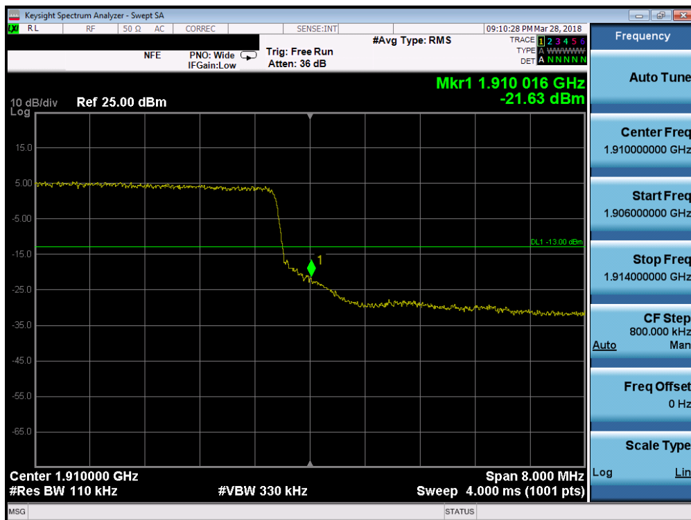
Plot 7-138. Upper Band Edge Plot (Band 2 - 10.0MHz QPSK - Full RB Configuration)
