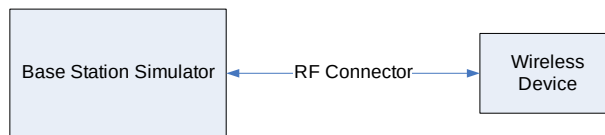
Figure 9-1 Power Measurement Setup
