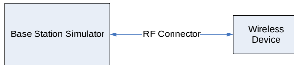
Figure 9-2 Power Measurement Setup
