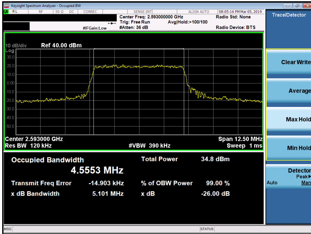
Plot 7-82. Occupied Bandwidth Plot (Band 41 - 5.0MHz QPSK - Full RB Configuration)
