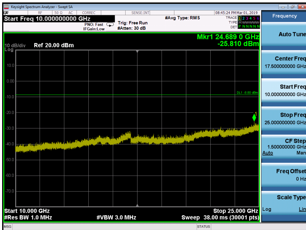
Plot 7-37. Conducted Spurious Plot (Bluetooth, 3Mbps – Ch. 0)
