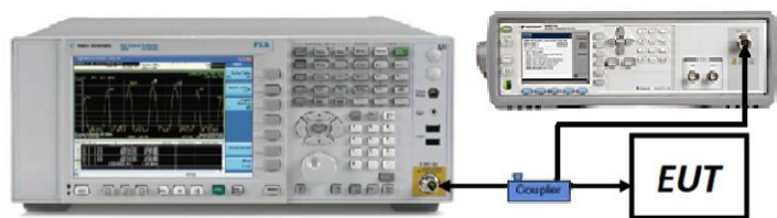
Figure 7-5. Test Instrument & Measurement Setup
