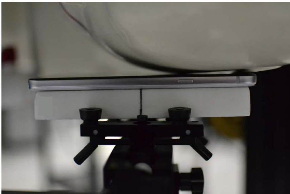
SAR Test Setup Photo 3 – Left Cheek
