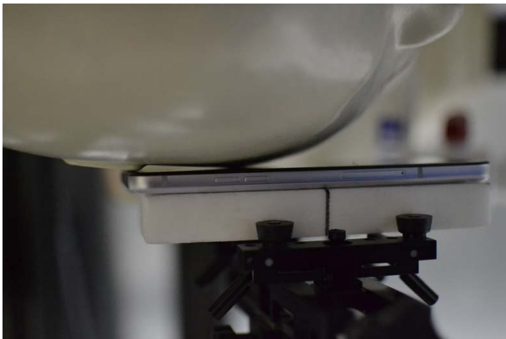
SAR Test Setup Photo 1 – Right Cheek
