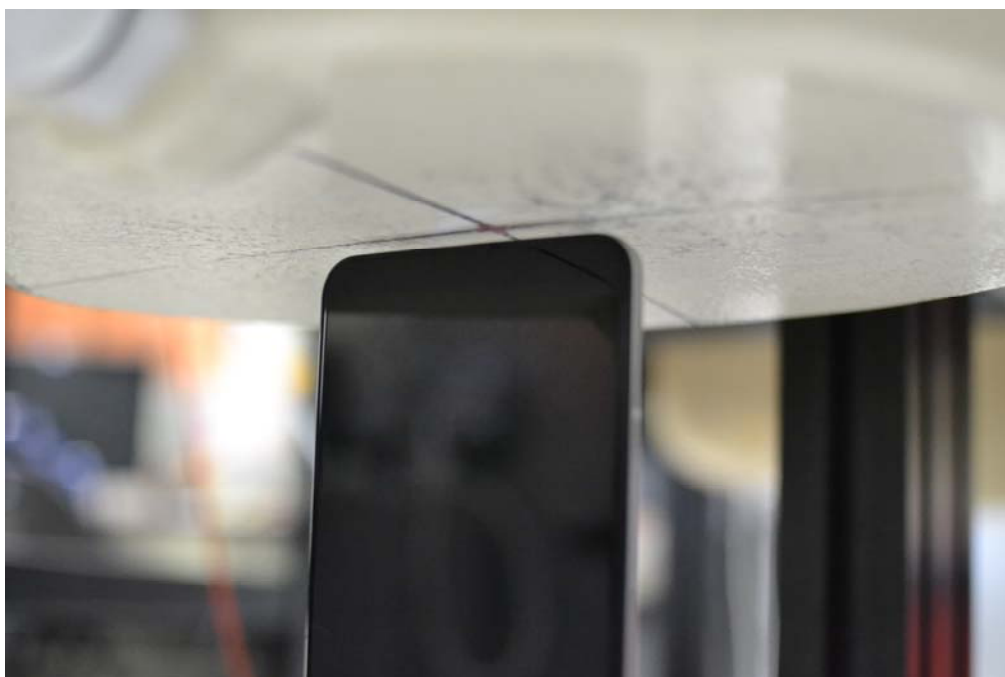
SAR Test Setup Photo 14 – Bottom Edge at 0.3cm
