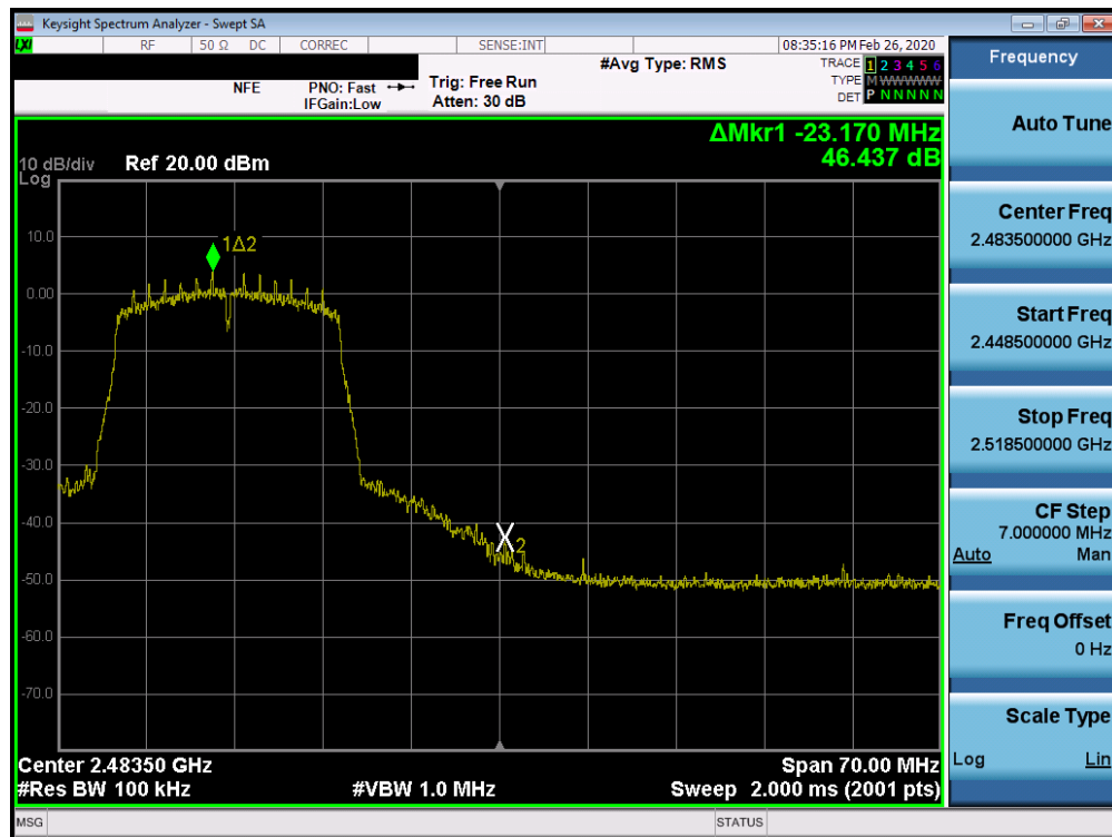
Plot 7-24. Band Edge Plot (802.11n (2.4GHz) – Ch. 11)
