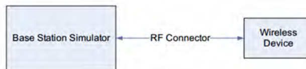
Figure 9.1 Power Measurement Setup
