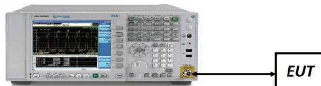
Figure 7-5. Test Instrument & Measurement Setup
