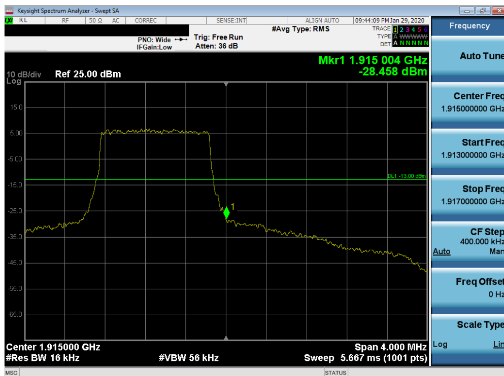
Plot 7-225. Upper Band Edge Plot (Band 25 - 1.4MHz QPSK - Full RB Configuration)
