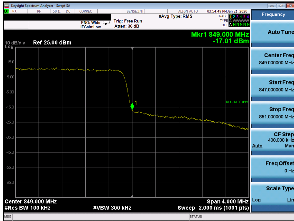
Plot 7-178. Upper Band Edge Plot (Band 26/5 - 3.0MHz QPSK - Full RB Configuration)
