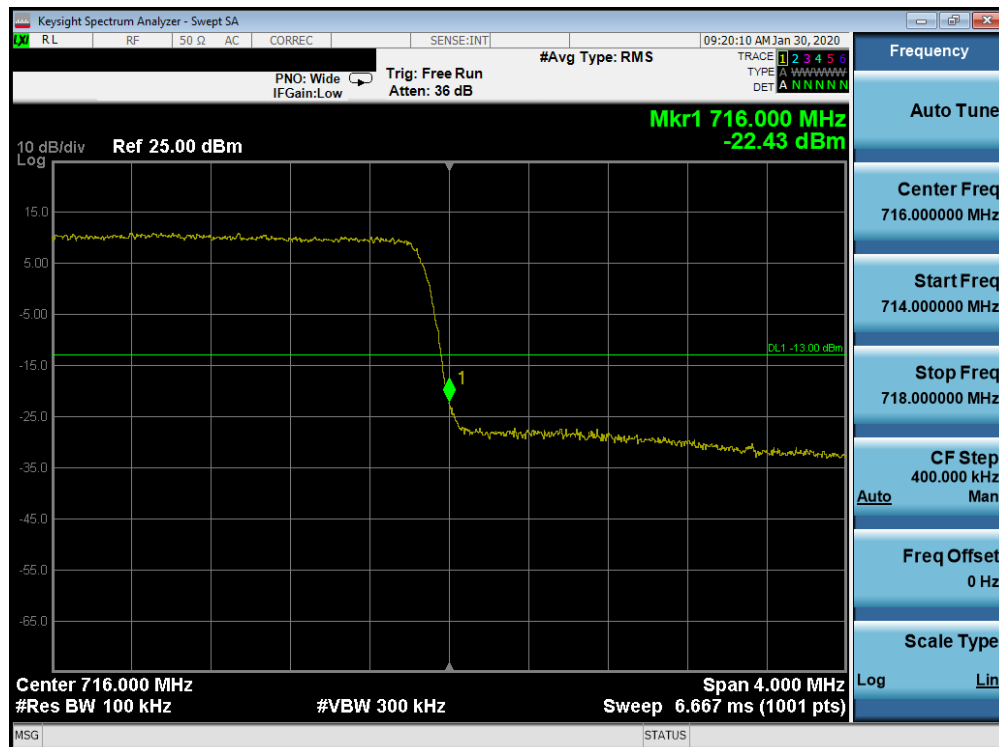
Plot 7-165. Upper Band Edge Plot (Band 12 - 3.0MHz QPSK - Full RB Configuration)
