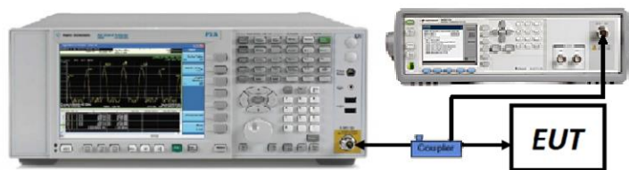
Figure 7-5. Test Instrument & Measurement Setup
