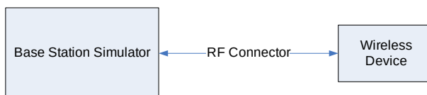
Figure 9-3 Power Measurement Setup
