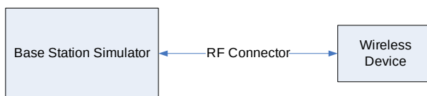
Figure 9-2 Power Measurement Setup
