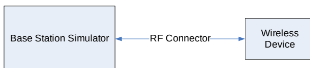
Figure 9-1 Power Measurement Setup
