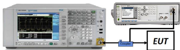
Figure 7-6. Test Instrument & Measurement Setup
