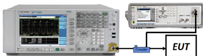
Figure 7-7. Test Instrument & Measurement Setup
