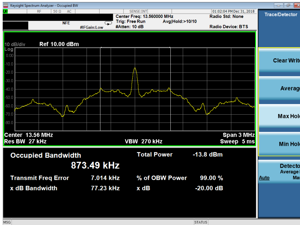
Figure 7-2. 20dB Bandwidth Plot
