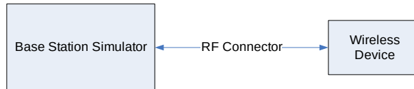
Figure 9-1 Power Measurement Setup
