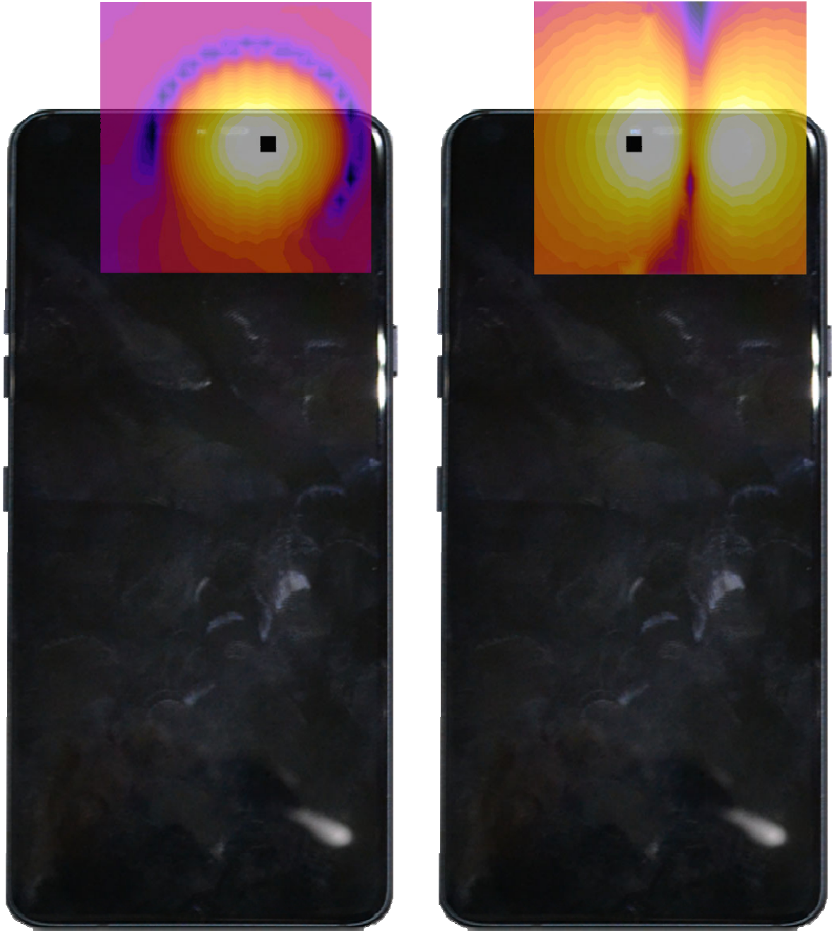
Figure 16-3 T-Coil Scan Overlay Magnetic Field Distributions
