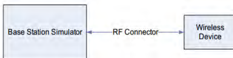
Figure 10.2 Power Measurement Setup
