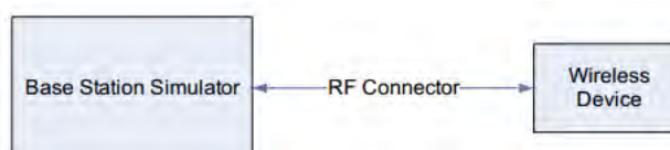
Figure 10.1 Power Measurement Setup
