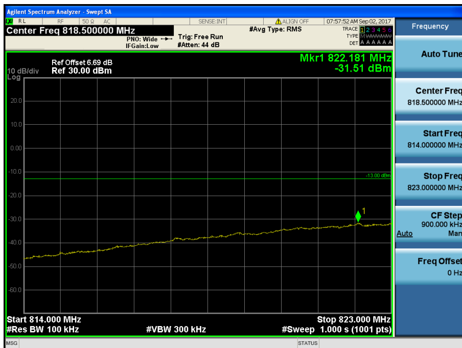
LTE Band 5 / 10MHz / 64QAM - RB Size/Offset (25/0)
