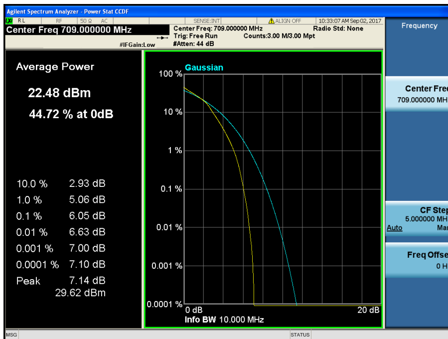
LTE Band 17 / 10 MHz / 16QAM - RB Size 50
