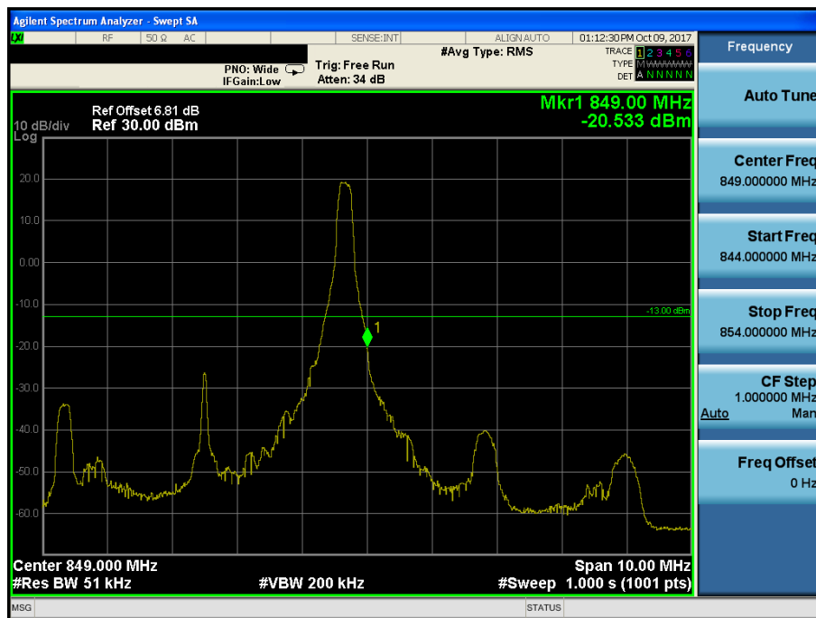
LTE Band 5 / 5MHz / 16QAM - RB Size/Offset (1/24)
