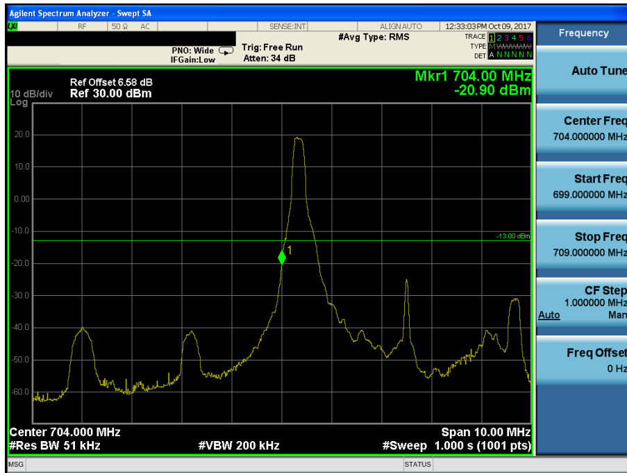
LTE Band 17 / 5MHz / 16QAM RB Size/Offset (1/0)
