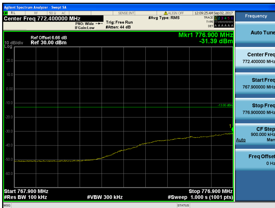
LTE Band 13 / 10MHz / 64QAM - RB Size/Offset (25/0)
