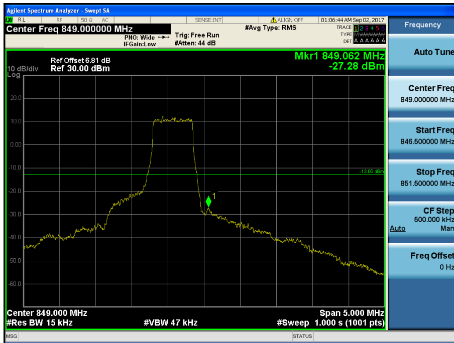
LTE Band 5 / 1.4MHz / QPSK - RB Size/Offset (3/3)
