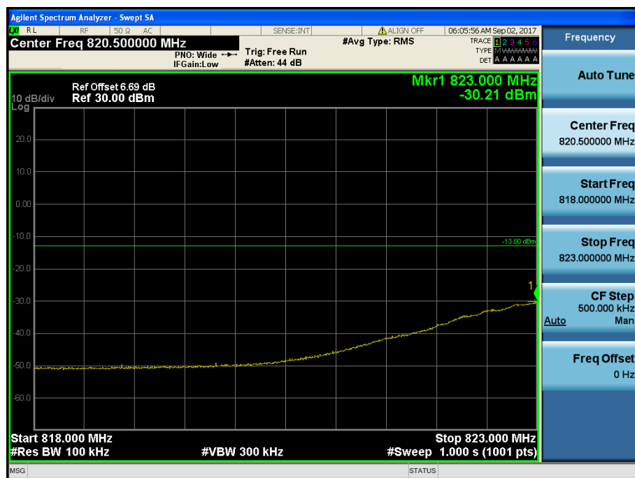
LTE Band 5 / 1.4MHz / 64QAM - RB Size/Offset (6/0)
