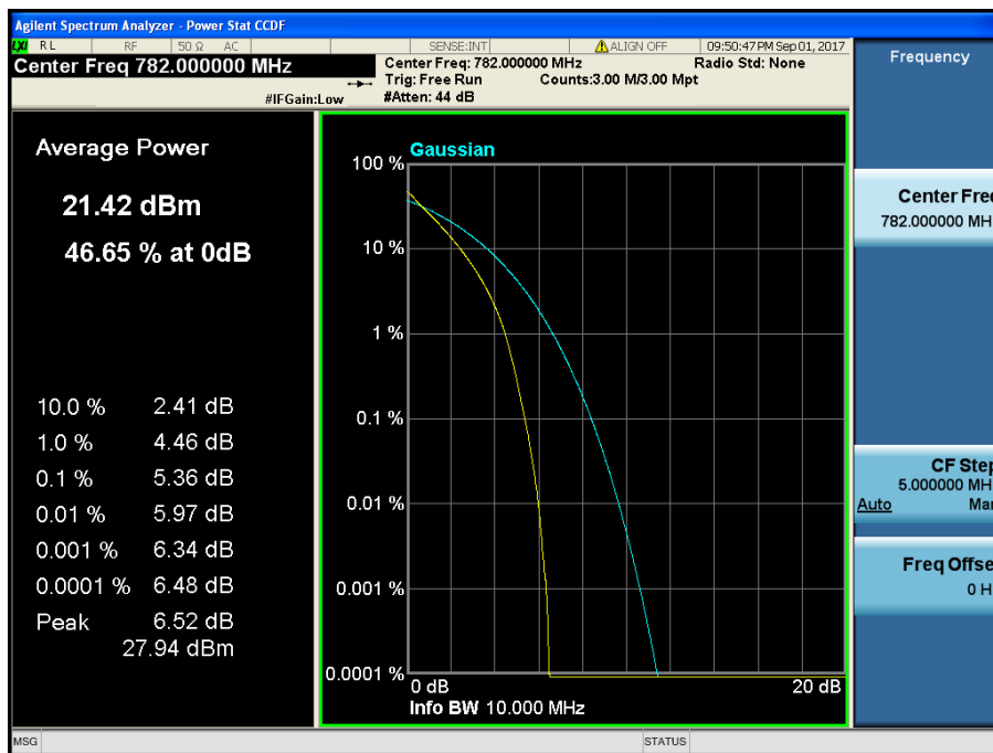
LTE Band 13 / 10 MHz / QPSK - RB Size 50
