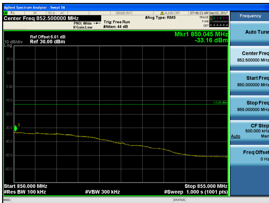
LTE Band 5 / 5MHz / 64QAM - RB Size/Offset (25/0)
