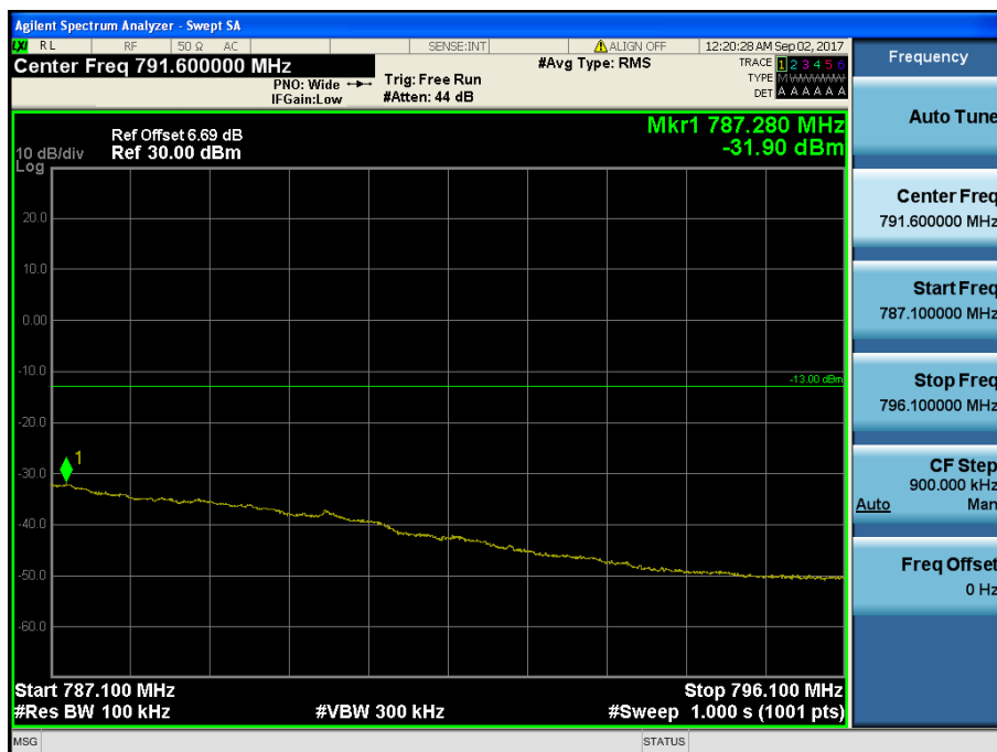
LTE Band 13 / 10MHz / 64QAM - RB Size/Offset (25/25)
