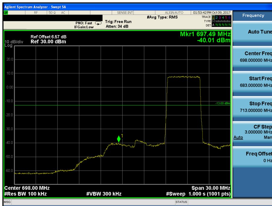
LTE Band 17 / 5MHz / QPSK RB Size/Offset (25/0)
