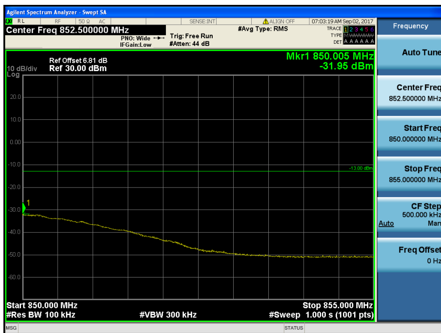
LTE Band 5 / 3MHz / 64QAM - RB Size/Offset (8/7)
