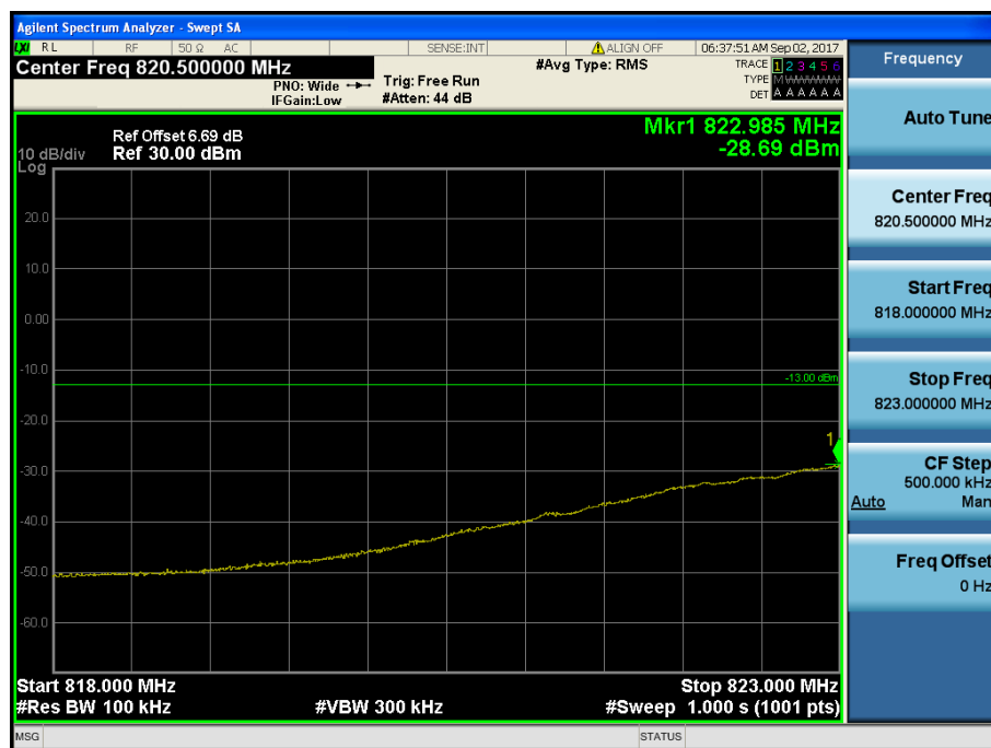
LTE Band 5 / 3MHz / 64QAM - RB Size/Offset (8/0)
