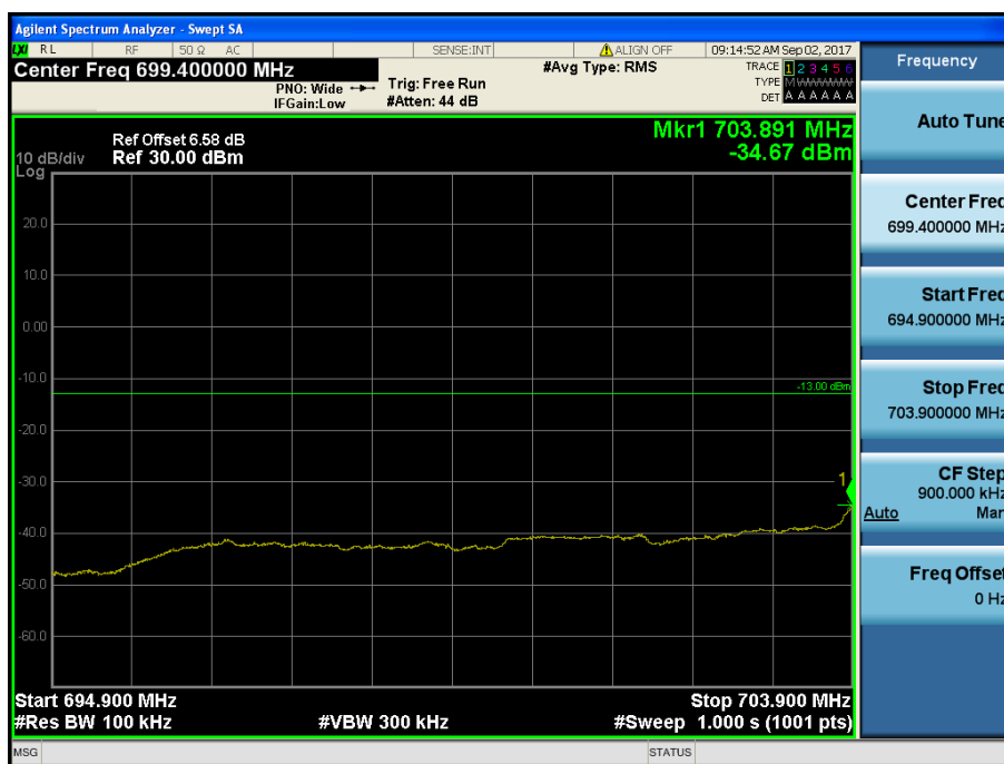
LTE Band 17 / 10MHz / QPSK - RB Size/Offset (25/0)
