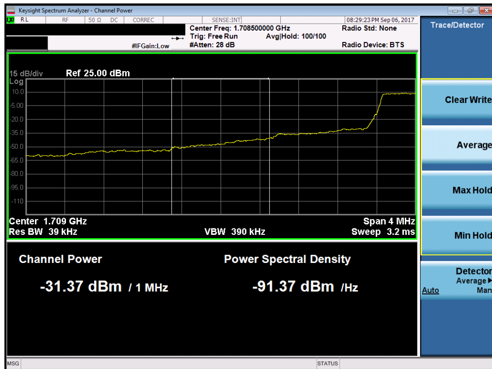
Plot 7-127. . Lower Extended Band Edge Plot (Band 4 – 1.4MHz QPSK - Full RB Configuration)
