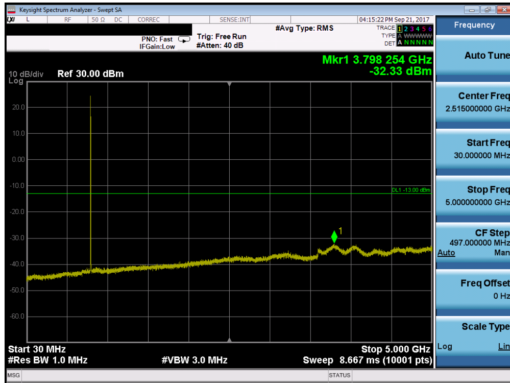
Plot 7-17. LTE Band 26 Conducted Spurious Plot (5MHz QPSK – RB Size 1, RB Offset 0 – Low Channel)
