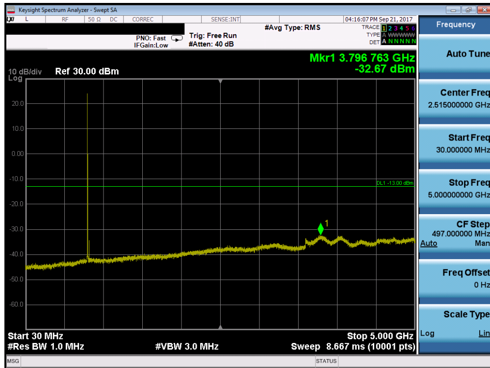
Plot 7-19. LTE Band 26 Conducted Spurious Plot (5MHz QPSK – RB Size 1, RB Offset 0 – High Channel)
