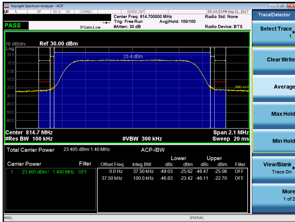
Plot 7-23. LTE Band 26 Channel Edge Plot (1.4MHz QPSK – RB Size 6– Low Channel)
