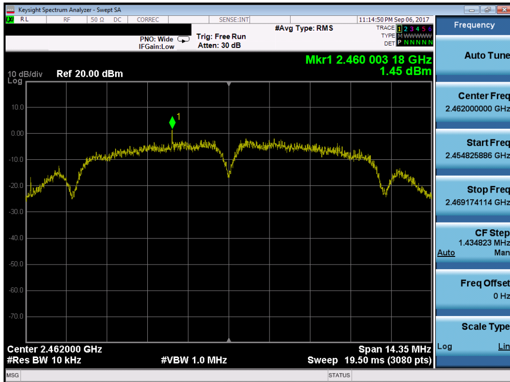
Plot 7-12. Power Spectral Density Plot (802.11b – Ch. 11)
