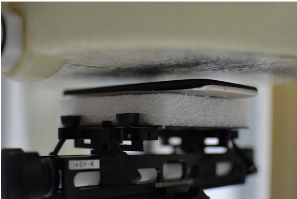
SAR Test Setup Photo 6: Front at 1.0 cm
