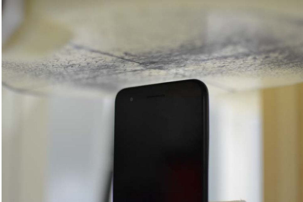
SAR Test Setup Photo 7: Top at 1.0 cm
