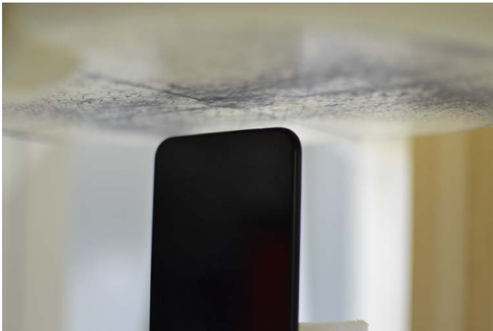
SAR Test Setup Photo 8: Bottom at 1.0 cm
