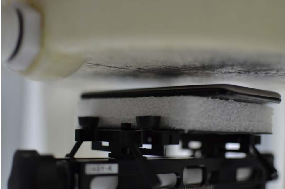
SAR Test Setup Photo 5: Back at 1.0 cm
