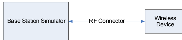
Figure 9-3 Power Measurement Setup
