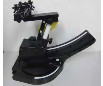
Figure E.6.1 Mounting Device
