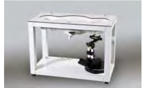
Figure E.5.1 SAM Twin Phantom
