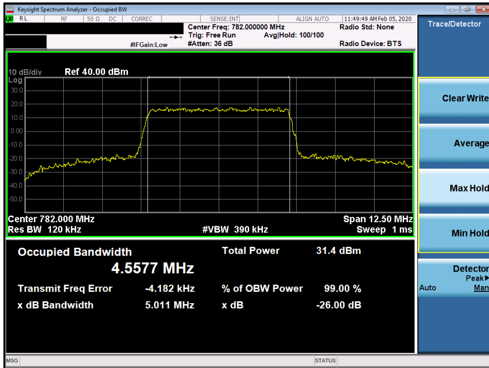
Plot 7-27. Occupied Bandwidth Plot (Band 13 - 5.0MHz 64-QAM - Full RB Configuration)
