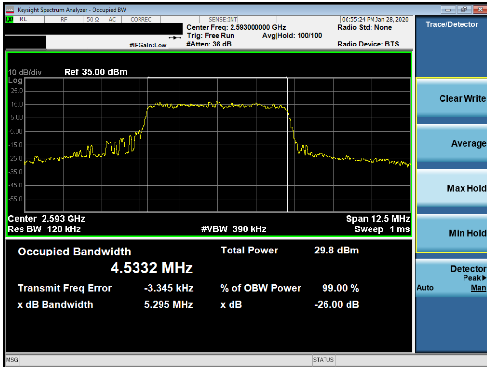
Plot 7-84. Occupied Bandwidth Plot (Band 41 (PC2) - 5.0MHz 64-QAM - Full RB Configuration)
