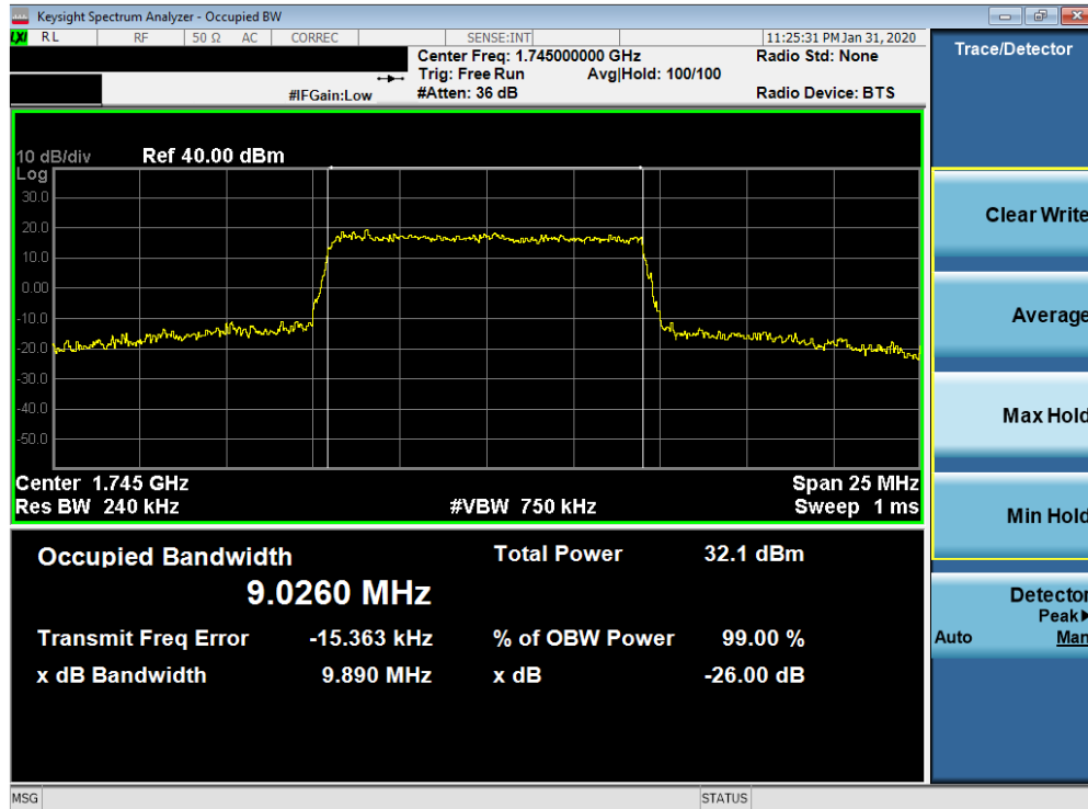
Plot 7-56. Occupied Bandwidth Plot (Band 66/4 - 10.0MHz 16-QAM - Full RB Configuration)
