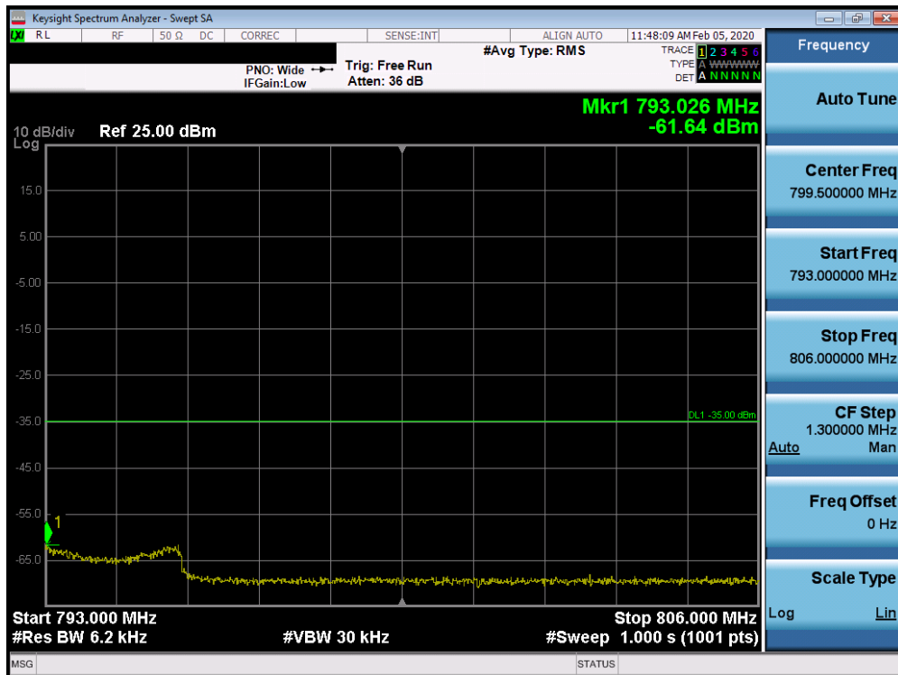
Plot 7-174. Upper Emission Mask Plot (Band 13 - 10.0MHz QPSK - Full RB Configuration)
