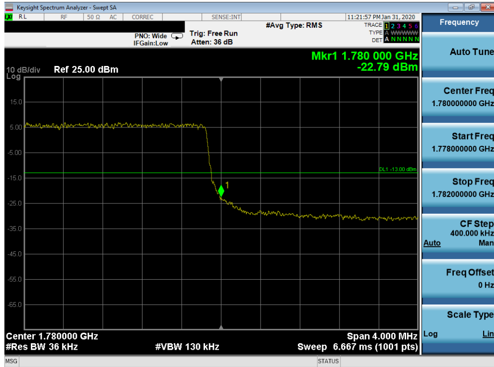
Plot 7-195. Upper Band Edge Plot (Band 66 - 3.0MHz QPSK - Full RB Configuration)
