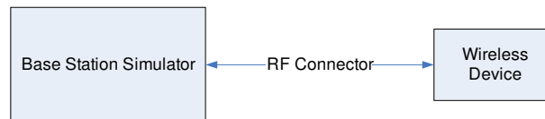
Figure 9-2 Power Measurement Setup
