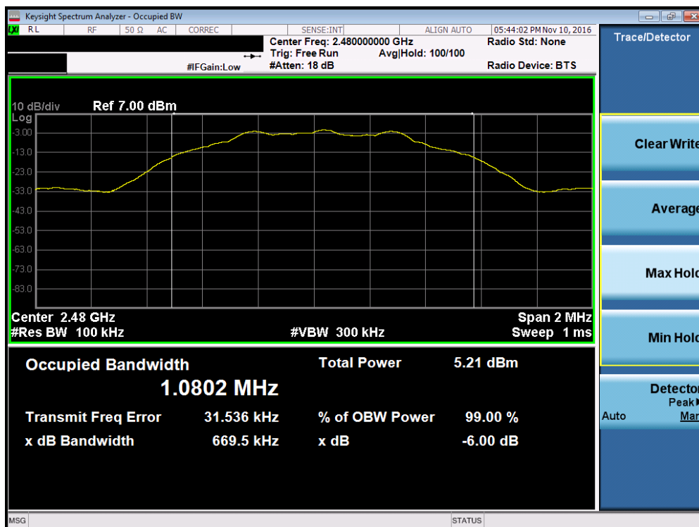
Plot 7-3. 6dB Bandwidth Plot (Bluetooth (LE) – Ch. 39)
