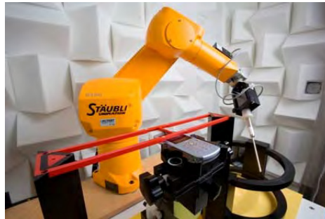
Figure 4-3 SPEAG Robotic System
