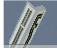
Figure 4-1 E-field Free-space Probe
