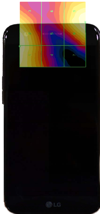
Figure 17-4 E-Field WD Scan overlay
