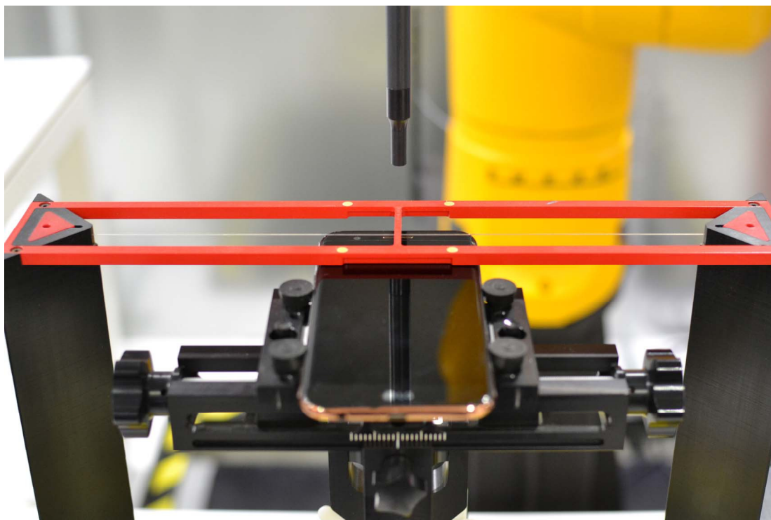
Figure 17-1 Ear Reference Point HAC Phantom Alignment
